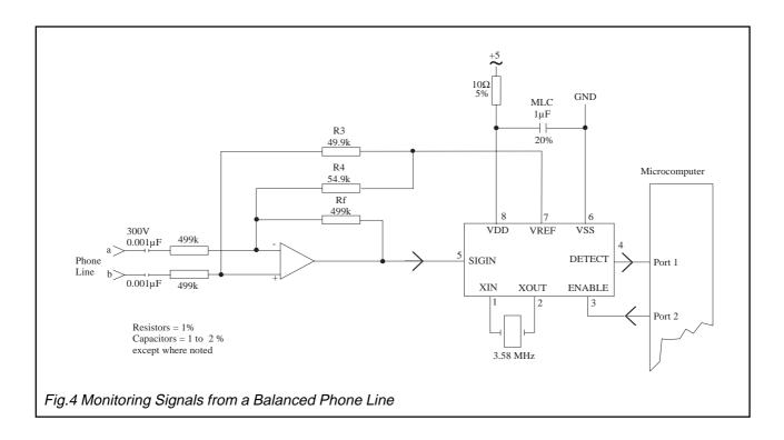
The minimum level required by the CMX673 is -38dBm. In general to optimise transient response and to limit spurious DETECTs, it is best to use the least sensitive configuration possible. However the gain of the buffer stage shown in Figure 4 may be varied to obtain the sensitivity required for a given application. The gain of this stage is equal to the ratio of Rf to Rin(-ve).
